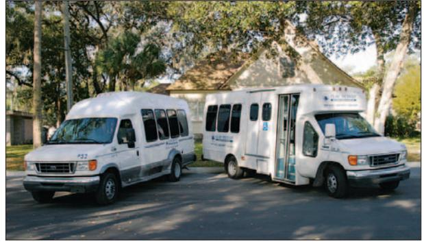
**Because 30% of Clay County's roads are unpaved, vehicles have a softer suspension, larger alternators and dual rear wheels.**
